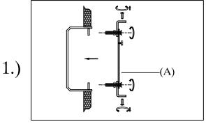
step1:Attach the mounting bracket to the outlet box by using two mounting screws.
