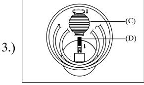
step3:Fix G9 LED on socket, and finally, attach the glass on socket.
