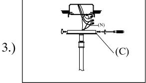
Step 3: Wire fixture to wires found in the electrical box. Install copper wire to mounting screw. Install fixture to mounting bracket, and tighten screws on the sides of the canopy to secure.
