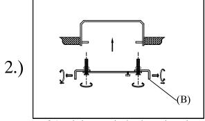
step2:Attach the mounting bracket to the outlet box by using two mounting screws.
