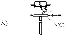
Step 3: Wire fixture to wires found in the electrical box. Install copper wire to mounting screw. Install fixture to mounting bracket, and tighten screws on the sides of the canopy to
