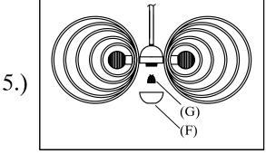
step5:Fix MR11 bulb on socket, and finally, secure the round cap tightly.
