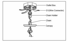
3. Wire fixture wire leads to outlet box wires. Wire copper ground wire from fixture to ground from outlet box. Pull canopy and screw ring up chain to ceiling and tighten securely.
