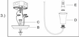
Step3:Install top loop to center stem and attach appropriate amount of chain to loop to achieve desired mounting height. Thread wire through every 3rd loop of chain.Remove ring from loop and slide down chain. Place canopy onto chain and let slide to top of fixture. Install nipple and cross bar into top of chain loop. Wire fixture to wires in outlet box. Copper wire is for Ground. Pull canopy through screw ring up chain to ceiling and tighten securely.
