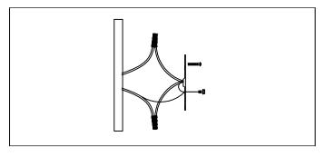
1. Remove mounting bracket from fixture and install to electrical box
