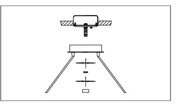
3. Install fixture to outlet box using hex nut and center finial lock up.
