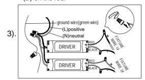
Step.3: Wire fixtures to red wires of the driver, wire black and white wire of the driver to wires in outlet box. Copper wire is for ground.
