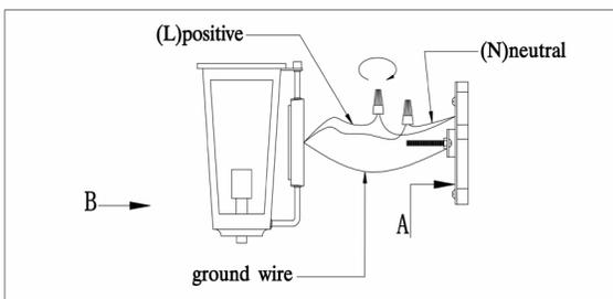
Step.2: Attach back plate to mounting bracket and tighten ball nuts so fixture meets wall. Caulk fixture where back plate meets the wall with silicone sealant. Leave a small gap at the bottom to let moisture escape.
