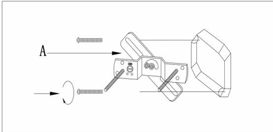
Step.1: Remove mounting bracket from fixture(B) and install to electrical box. then wire fixture to wires in outlet box. Copper wire is for Ground.
