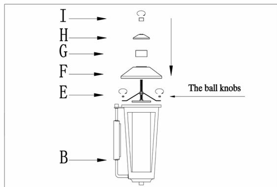
Step.4: Attach trestle(E) to fixture , using ball knob at screws. Then the hood(F), neck(G), top cover(H) through the threaded tube. Then tighten the finial(I).
