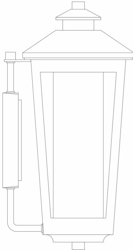
To prevent water intrusion, caulk around back-plate where fixture meets the wall using outdoor silicone sealant. Leave a small gap at the bottom to allow moisture to exit.
