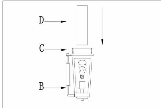
Step.3: Slide four clear glass(C) into fixture(B), install MB bulb and then slide frosted glass(D) into fixture(B).
