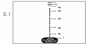
Step. 2: Run wire through stems(B)and combine stem lengths to meet desired mounting height.
