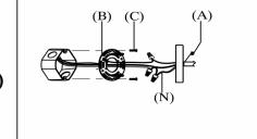
step2: Wire fixture to wires in outlet box. Copper wire is for Ground. Attach wall sconce to mounting bracket and tighten ball nuts (A) so fixture meets wall.
