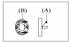
step1: Remove mounting bracket (B) from fixture and install to electrical box using mounting screws (C).
