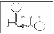
step3: Loosen the lock screws (D). Install E12 bub(E) and attach glass (F). Secure glass (F) by tightening lock screws (D).
