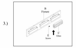
Step.3: Attach glass (C) to fixture (B) using screws (E).
