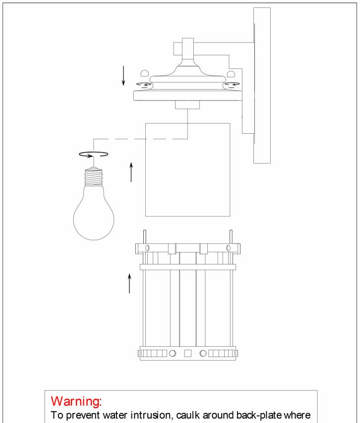
fixture meets the wall using outdoor silicone sealant.
