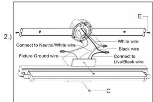
Step2:Wire fixture to wires in outlet box. Copper wire is for Ground. Attach canopy to mounting bracket and tighten with ball nuts (C),Screws (E).
