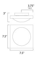
\*height from center of the outlet to the top of the fixture
