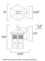
MEASUREMENTS DIMENSION BACK PLATE
