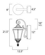
eight from center of outlet to the top of the fixture
