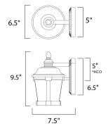
\*height from top of the fixture to the center of outlet
